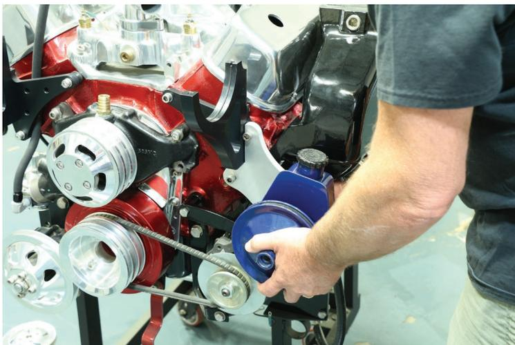
Put the pump on the bracket using the 3/8" hole and slot at the end of the bracket.
