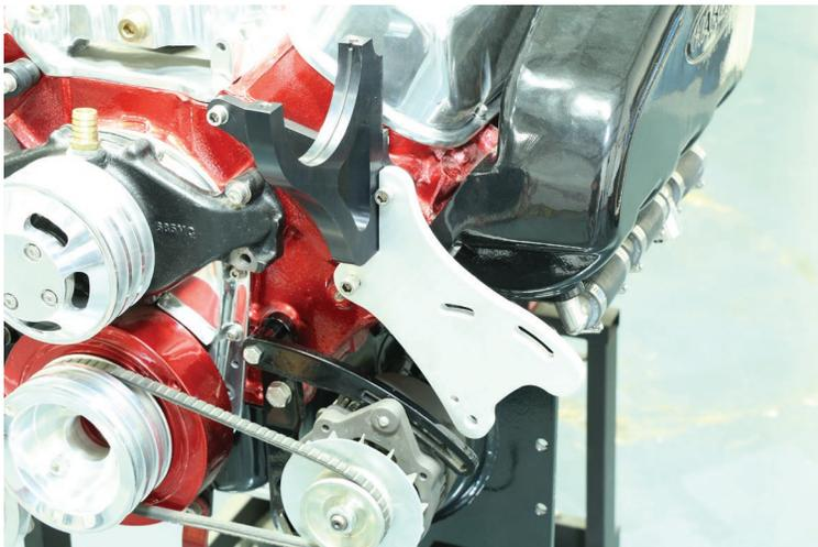
Attach bracket over the closed cooling tank port mount bracket using the 2 longer supplied bolts.
