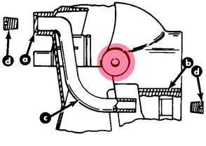
a - Gimbal Housing b - Bell Housing c - Water Hose d - Tapered Inserts
