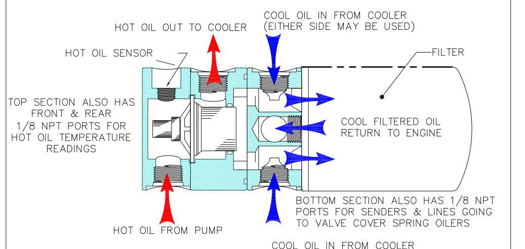
NOTE: BODY SECTIONS MAY BE ROTATED IN 90° INCREMENTS TO SUIT INSTALLATION.
