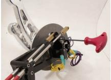
The shifter can be mounted to the side panel by either thru bolting with 1/4" x 1 1/4" flat head bolts and nuts or #14 x 1" oval head screws. Make sure that the shifter is mounted solid to the side panel and that the levers can operate freely without any interference. Follow the wiring diagrams below for the correct connections for each of the components.
