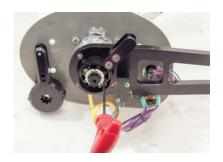
The neutral safety switch needs to be positioned so the connections point away from the shift cable connection as to not have any interference.
