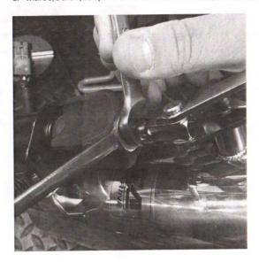
D. Reinstall replacement 3/8 square assembly, but do not tighten nut.
