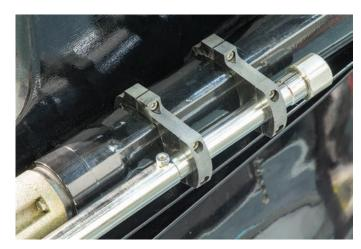
7. Remove pin from actuator. Cycle actuator several times and watch the actuator for smooth operation
