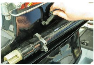
5. Butt end of push rod against trim pin cup at its centerline.
