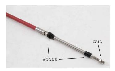
2. Slide tube end cap onto the cable with threaded opening facing the end of the cable. Replace rubber boots and cable nut.
