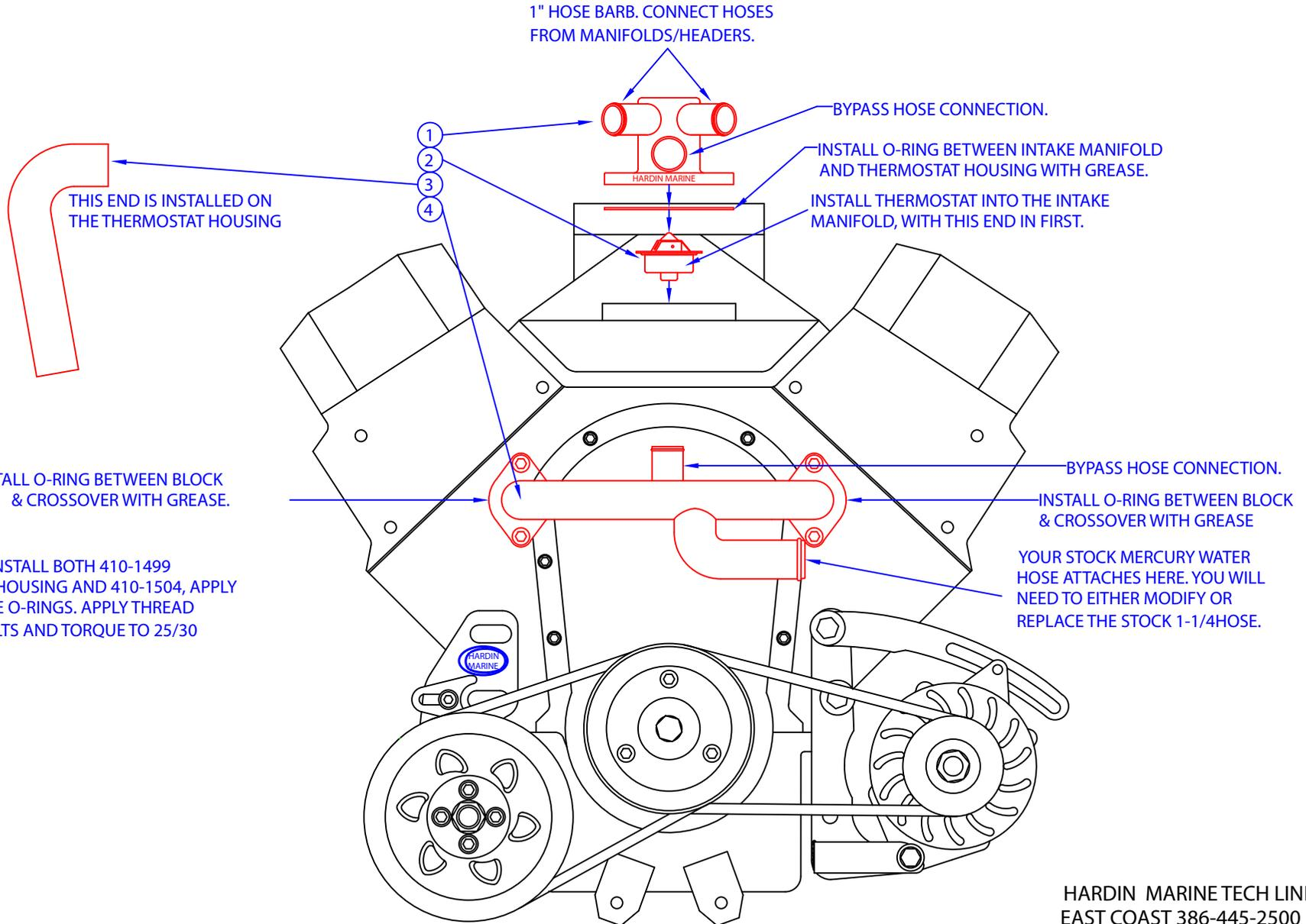
NOTE: WHEN INSTALL BOTH 410-1499 THERMOSTAT HOUSING AND 410-1504, APPLY GREASE TO THE O-RINGS. APPLY THREAD SEALER TO BOLTS AND TORQUE TO 25/30 FT. LBS..
