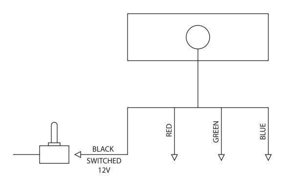
Black wire will always go to 12v. The Red, Green and Blue wires are always to ground if used. See color chart below for LED color wiring options.
