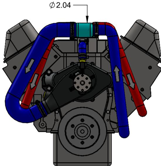
THIS IS A STANDARD RAW WATER THERMOSTAT HOUSING. THIS HOUSING ALLOWS WATER TO BE BYPASSED TO THE EXHAUST MANIFOLDS UNTIL THE THERMOSTAT OPENS. ONCE THE THERMOSTAT OPENS, ALL IN COMING WATER IS CIRCULATED THROUGH THE ENGINE BEFORE GOING OUT THE EXHAUST.
