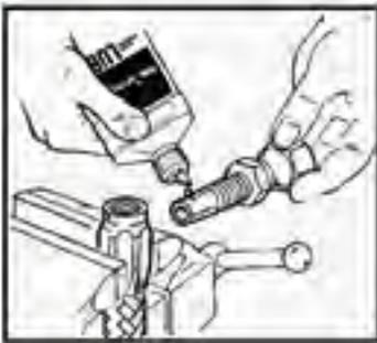
**MALE ENDS:** Push assembly tool into nipple.
