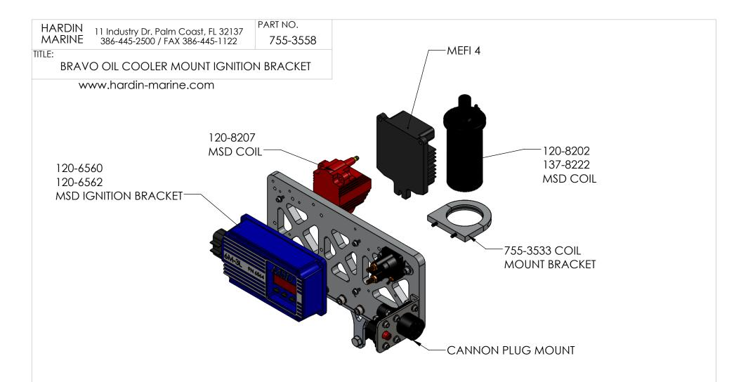
THESE ARE THE PARTS THAT CAN MOUNT TO THE BRACKET
