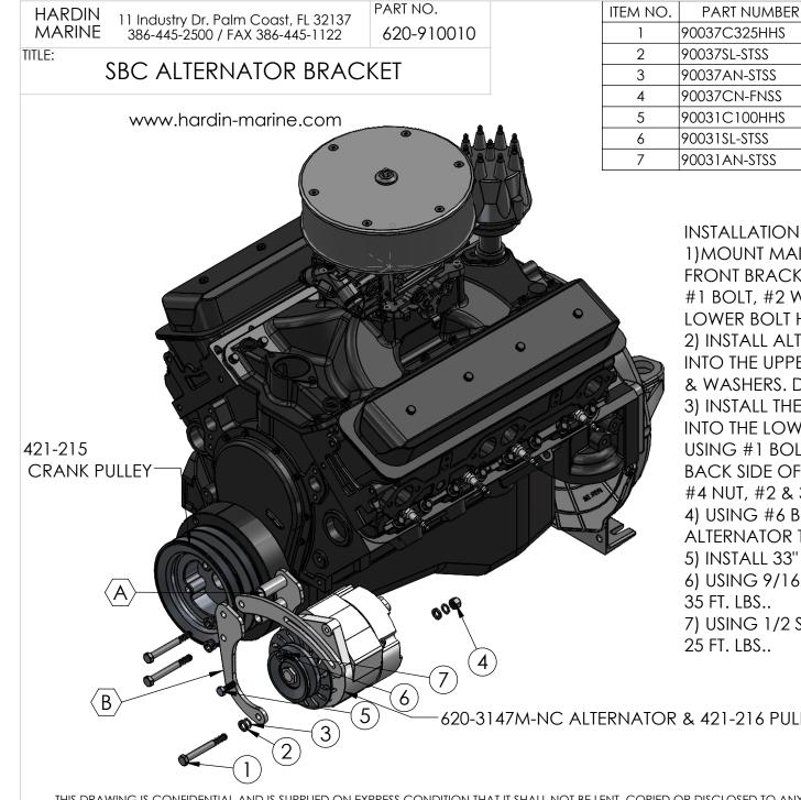
QTY. 90037C325HHS BOLT, 3/8-16 x 3.25 3 90037SL-STSS WASHER, LOCKING - 3/8 4 90037AN-STSS WASHER, 3/8 AN 4 NUT, 3/8-16 90037CN-FNSS 1 90031C100HHS BOLT, 5/16-18 x 1.00 1 90031SL-STSS WASHER, 5/16 LOCK 1 90031AN-STSS 1 WASHER, 5/16 AN INSTALLATION INSTRUCTIONS: 1) MOUNT MAIN BRACKET, FIG. A & THE FRONT BRACKET, FIG. B TO THE BLOCK USING #1 BOLT, #2 WASHER & 3 LOCK WASHER IN LOWER BOLT HOLE. DO NOT TORQUE. 2) INSTALL ALTERNATOR SWING ARM, FIG. C,
