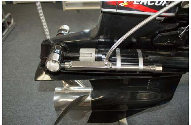
10. If replacing an existing cable system you can remove the cable from the thru hull and use the new center section in the old stainless housing.
