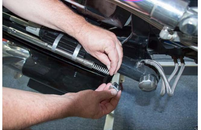
9. Install the sensor onto the actuator using the two 10/32 screws provided with the cable towards the back of the boat.
