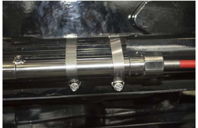
7. Remove pin from actuator. Cycle actuator several times and watch the actuator for smooth operation
