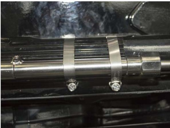
7. Remove pin from actuator. Cycle actuator several times and watch the actuator for smooth operation
