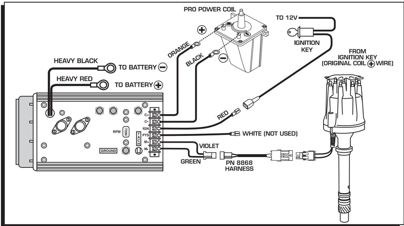
Figure 12 Wiring to an MSD 7ML-2 Ignition Control.
